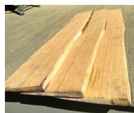
Each shingle is 3 ft. long. About a foot is exposed once installed.
